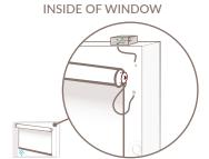
The J-Box can be located behind the drywall on either side of the window or within the window opening.
