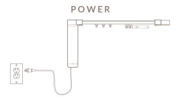
The Plug and Play motorized system uses a traditional 3 prong plug to draw power from a wall outlet. Each motor requires its own connection of 110 volt direct power.
